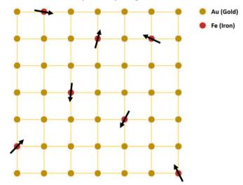
**Fig.2.** Schematic illustration of AuFe spin glass in which the iron atoms as magnetic impurities are mixed randomly to the nonmagnetic gold matrix. The spins associated with iron atoms represented by arrows are trapped in random directions.
